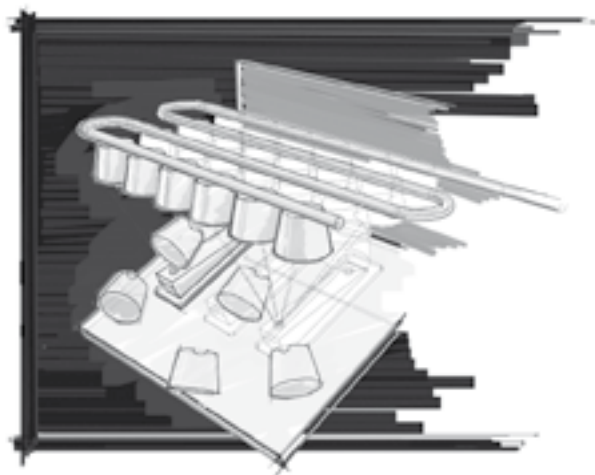
Horizontal ice evaporator and spray-system technology
