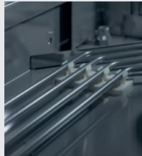
Stainless steel dosing pipes
