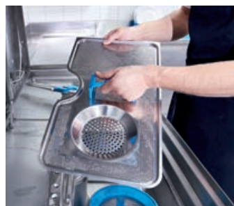
The blue operating concept: any parts that are blue can be removed, cleaned and replaced. For extra peace of mind, the M-iClean HXL automatically checks that you've put everything back in the right place.
