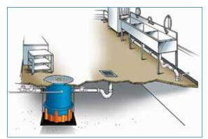
TZ-600 installed Indoors & Hanging Between Floors using HA-400/600. Shows optional FTCA-36 Aluminum Cover with 4" Brass Cleanout
