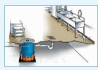
TZ-600 installed between floors using Hanging Assembly & FTCA-36
