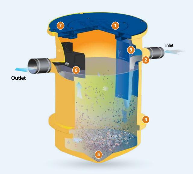
Solids-laden effluent from the kitchen flow is slowed and forced downward in a vertical baffle, where solids filter out of the flow and sink to the bottom of the solids storage area. The "cleaned" effluent flows through the outlet. Pumping the Trapzilla® Solids Separator is easy—the pumper removes the lid and vacuums out the solids.
